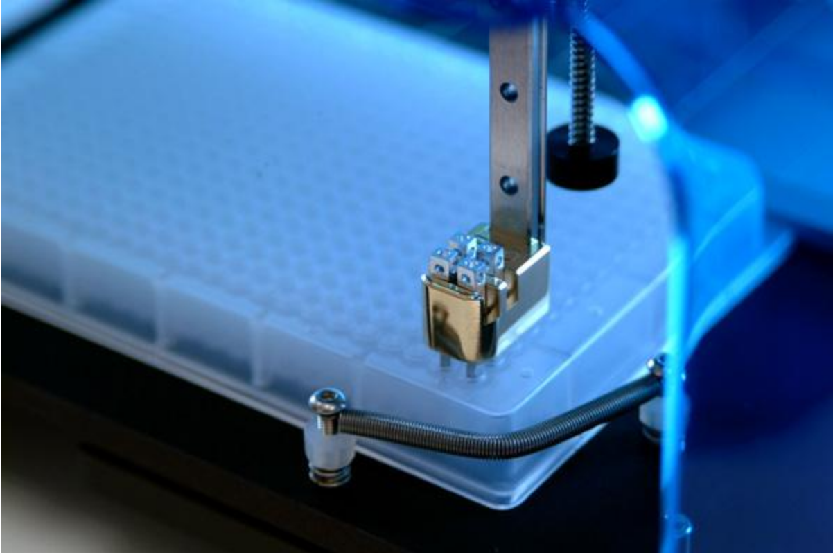
Figure 3. SpotBot®3 Microarrayer in the sample loading position. The Professional Series Printhead and 4 946MP4 Pins move into the loading position in the first group of 4 wells in the 384-well microplate. A loading time of 3 seconds allows each pin tip to load 0.2 \mu\text{l} of sample from each well containing 5 \mu\text{l} of total sample volume.
