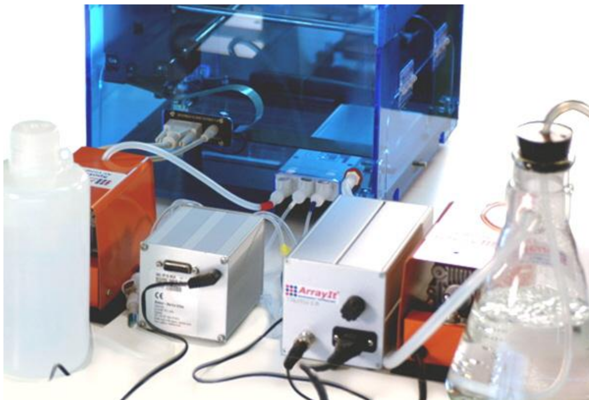
Figure 11. Shown is a photograph of the SpotBot ® 3 Personal Microarrayer including the accessories. The translucent wash buffer reservoir, orange air compressor for the dry station, silver peristaltic pump for the wash station, silver megasonic power supply and humidification system including the orange air compressor and humidification reservoir are shown correctly configured behind the instrument. The COM cable, power supply, dry station fitting (red), wash buffer fitting (white), waste buffer outtake (blue), and humidification tubing are shown correctly attached to the back of the instrument. The modular and compact accessories design improves system utility and performance and simplifies maintenance and repair. The SpotBot ® 3 Protein Edition Microarrayer is configured similarly except that the humidification is replaced by dehumidification (see Figure 9) and a chiller bath is added for deck cooling.
