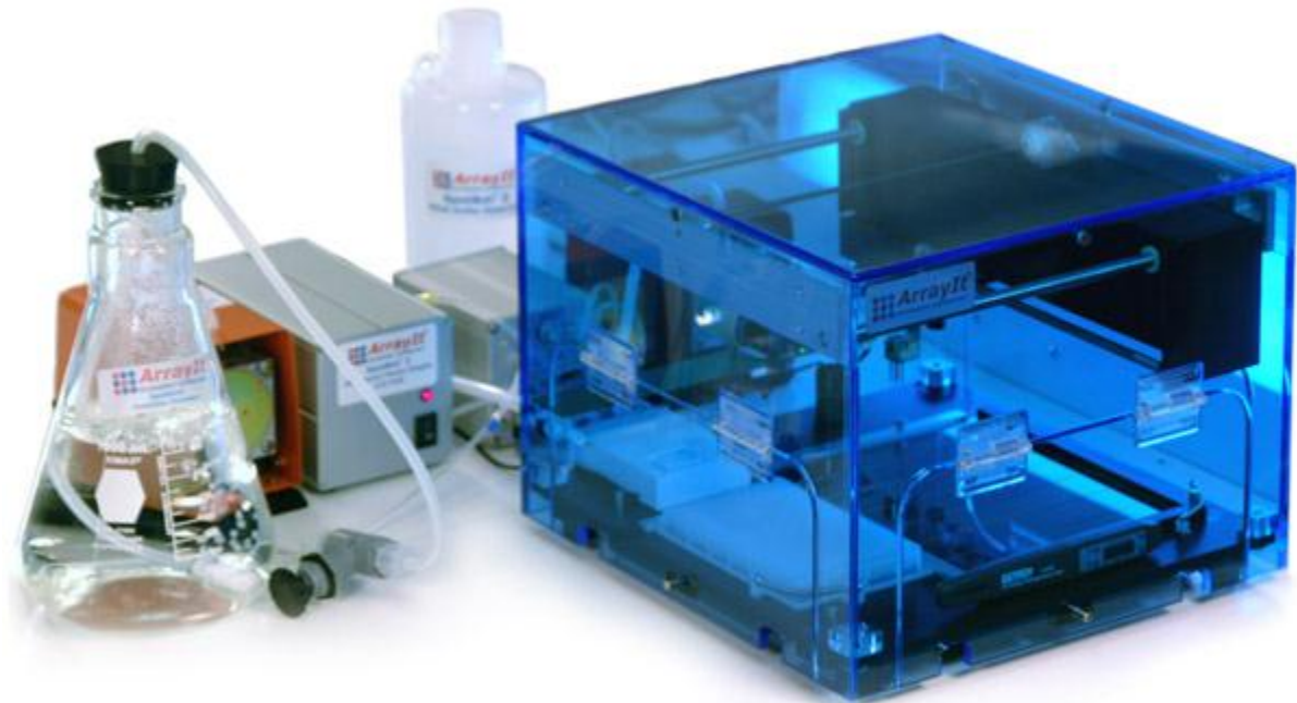
Figure 10. Shown is a photograph of the SpotBot ® 3 Microarrayer including the accessories. The translucent wash buffer reservoir, orange air compressor for the dry station, silver peristaltic pump for the wash station, silver megasonic power supply and humidification system including the orange air compressor, humidification reservoir and gray valve are shown correctly configured behind the instrument. The modular and compact accessories improve system utility and performance and simplify maintenance and repair. Inside the instrument, the microplate, L-bracket and temperature/humidity pen are visible. The SpotBot ® 3 Protein Edition Microarrayer is configured similarly except that the humidification is replaced by dehumidification (see Figure 9) and a chiller bath is added for deck cooling.
