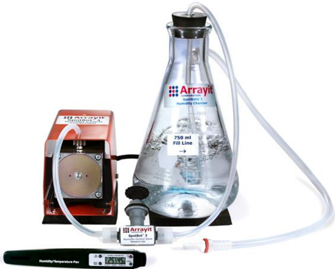
Figure 5. The Humidification System for SpotBot ® 3 Personal Microarrays includes a Humidity Control Compressor, Control Valve, Humidity Chamber, and Temperature and Humidity Pen. The system allows humidification of the internal instrument chamber from ambient to 80% relative humidity (RH) with an accuracy of \pm 1\% . The same core components and instrument port are used for the Dehumidification Apparatus (see Fig. 9).
